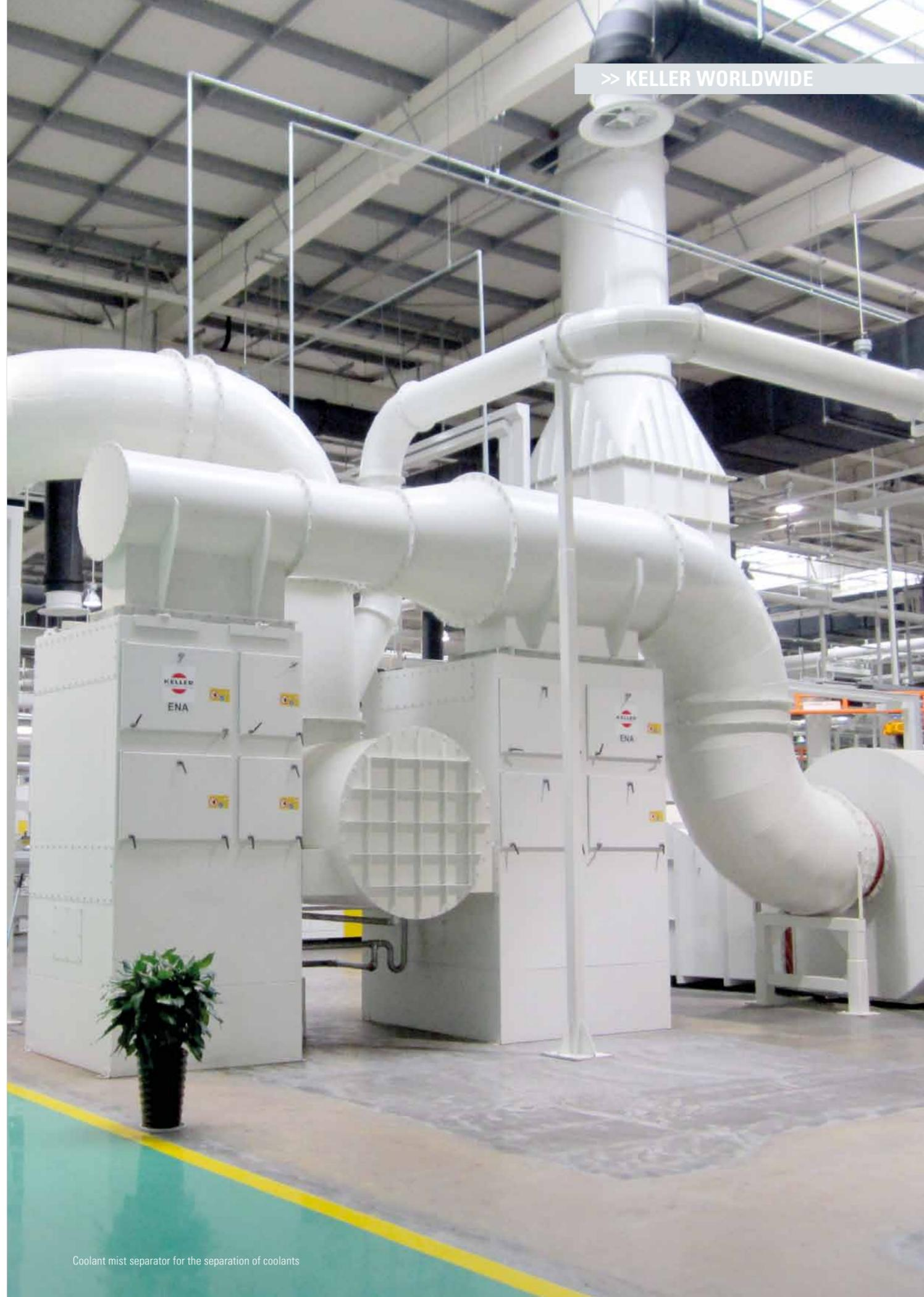
Coolant mist separator for the separation of coolants
