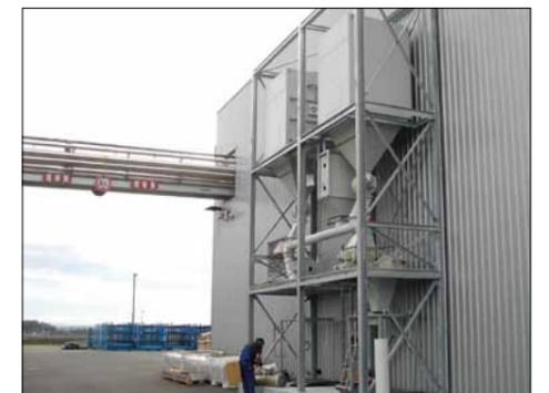
Dry separation VARIO 4 with briquetting system
