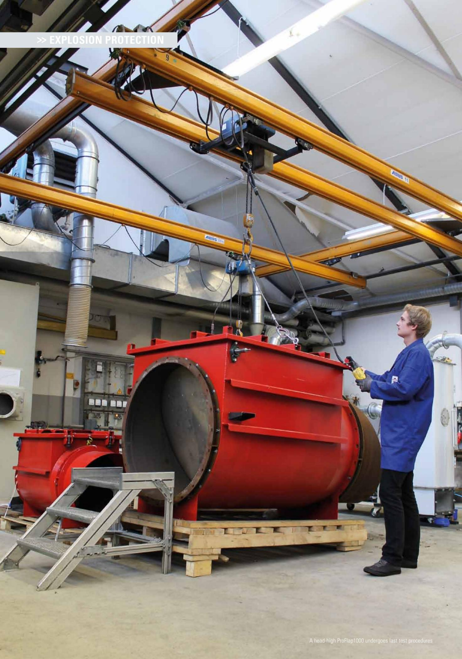
A head-high ProFlap1000 undergoes last test procedures
