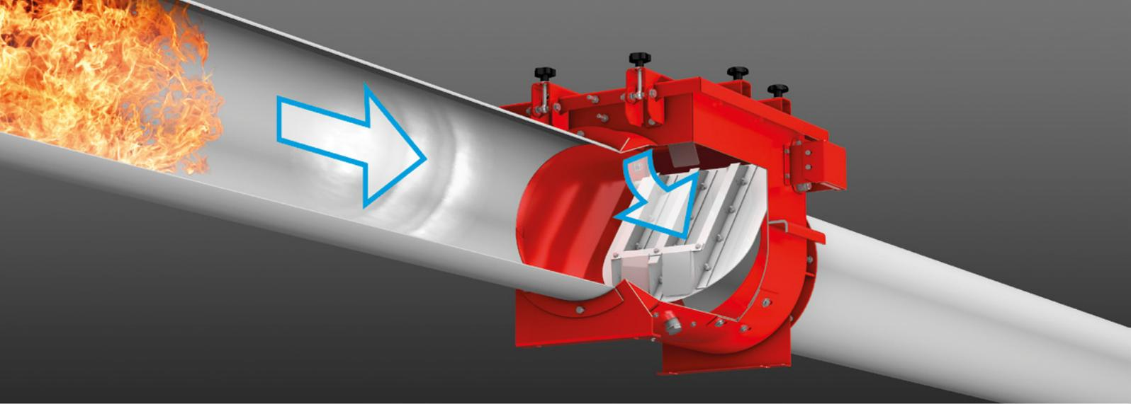
ProFlap back pressure flap avoids the spreading of explosion pressure and flame into the workroom.
