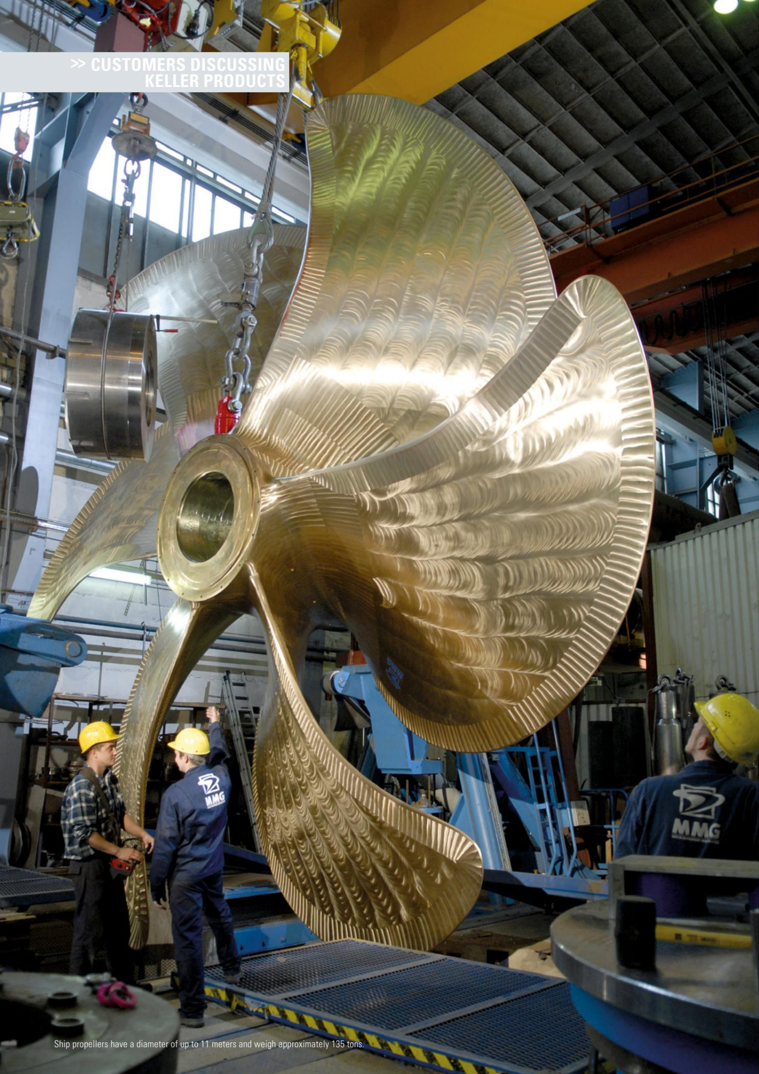
Ship propellers have a diameter of up to 11 meters and weigh approximately 135 tons.
