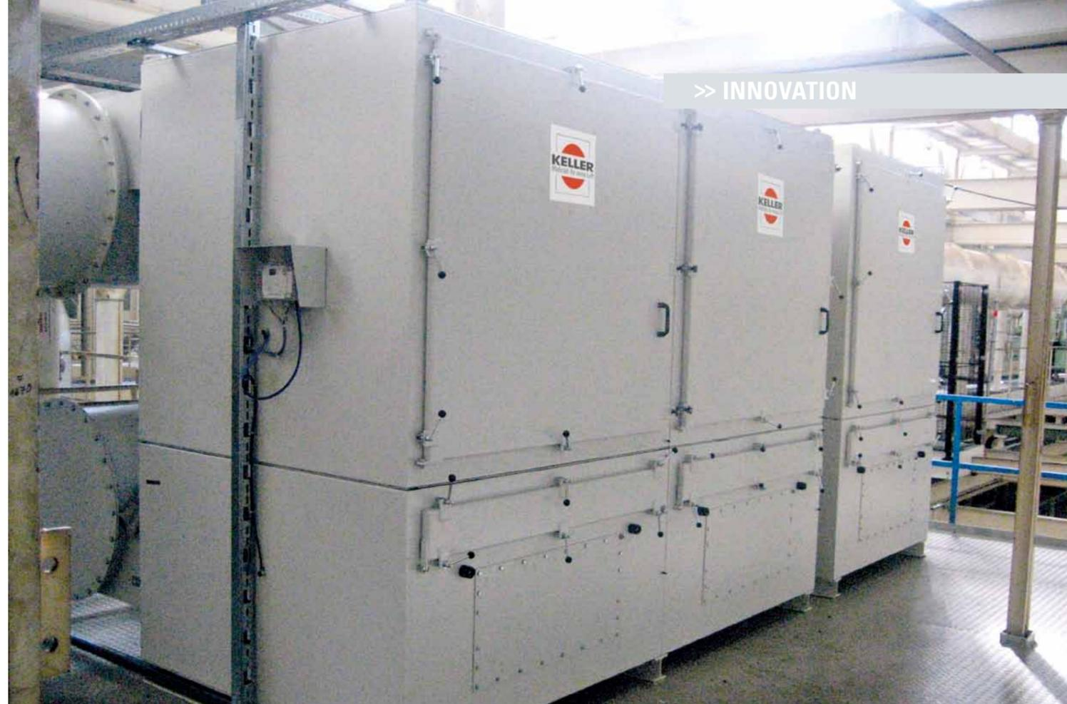
AERO reliably separates coolant aerosols which are created during the grinding of automotive parts.
