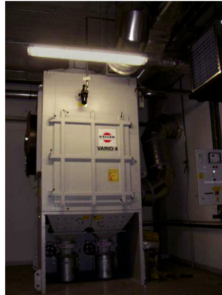
Decentralized filter with flameless pressure discharge
