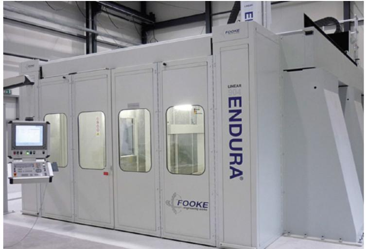
Portal Milling machine with enclosure
