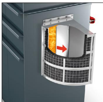
Constructive explosion protection through harmless relief of explosion pressure. Q-Box is a flameless pressure relief system with a burst disk and metal mesh for rapid heat reduction.
