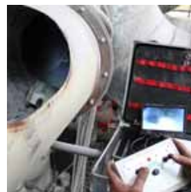
Robot cams help getting an insight into sections which otherwise would not be visible
