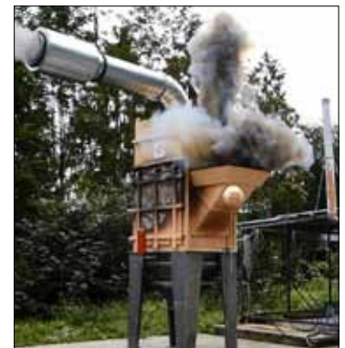
Explosion suppressed by ProPipePlus
