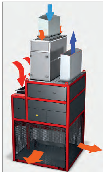
Example A: The cleaned process exhaust air and outdoor air are heated on demand and combined with ambient air inside the plant.
